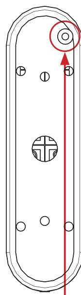
Anti-tamper photocell. To activate the function, please refer to page 16 «Anti-tamper function»
